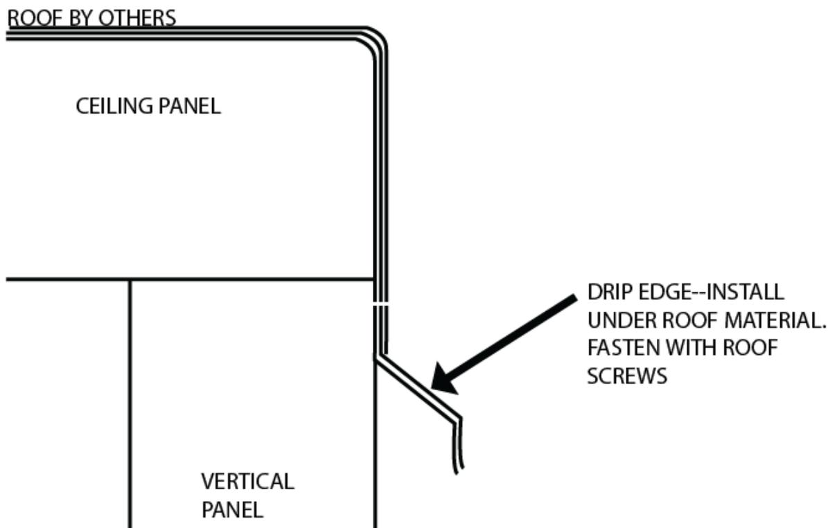
NOTE: INSTALL CORNER PIECES. THEN STRAIGHT RUNS. OVER FELT PAPER BEFORE INSTALLING WEATHER ROOF. DRIP EDGE PIECES. CAN OVERLAP CORNER PIECES AND EACH OTHER BY 1½" MAXIMUM. SOME TRIMMING BY INSTALLER MAY BE REQUIRED.
